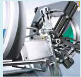
Fitted counter-pressure unit
