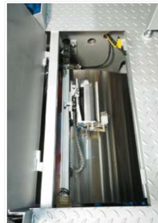
Access to central drum for cleaning
