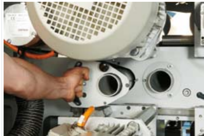
Disassembling of the intercolour dryers
