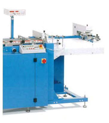
Hook-on and swivelling chute delivery S 500 with infinitely-variable drive.
