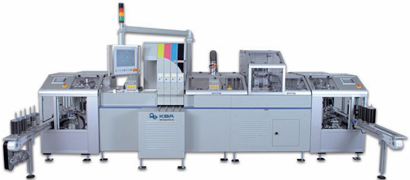
Complete CD-Print system with four print stations, feed and delivery compacts on a very small footprint
