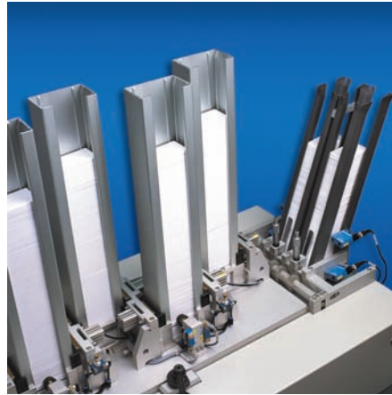
Loading magazine module (right) and four additional card holds for large print runs significantly reduce the need for reloading
