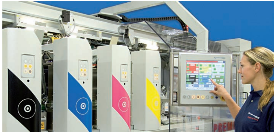
The control panel with a user-friendly touch screen can be pivoted around the whole machine to make things as easy as possible for the operator
