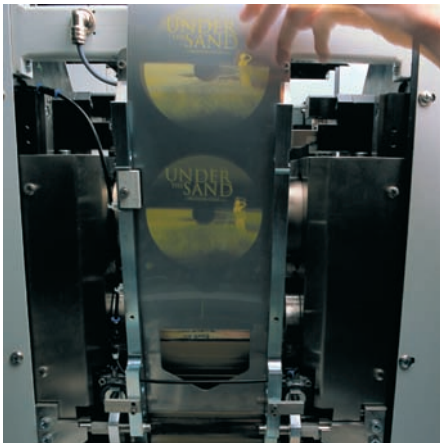
Semi-automatic printing plate replacement ensures high registration accuracy and takes no more than 5 minutes. You can use analogue or digital waterless printing plates
