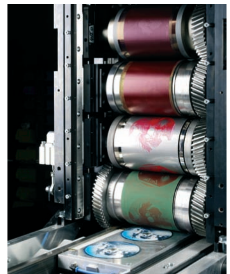
Short inking technology used on the Premius delivers photorealistic offset quality
