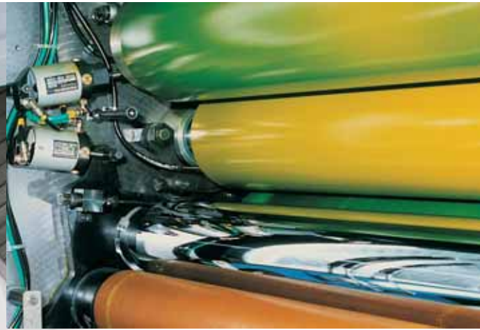
The cylinders are seated in zero-play bearings in rigid side-frames
