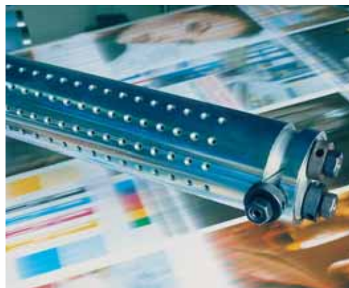
Cantilevered turner bars make for easy handling
