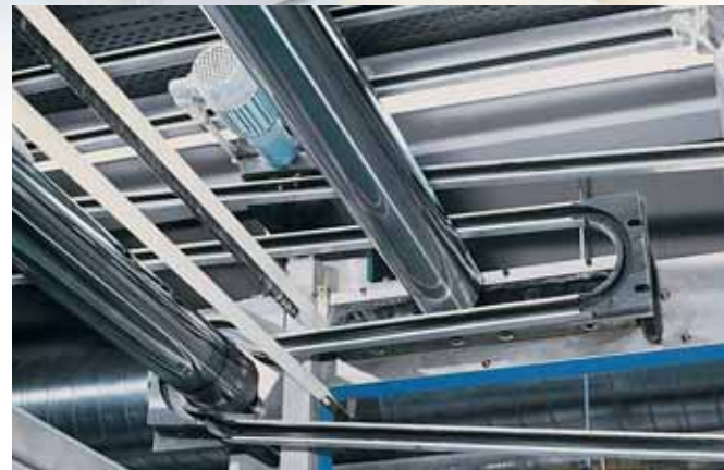
The automatic webbing-up chain threads the web into the press – fast
