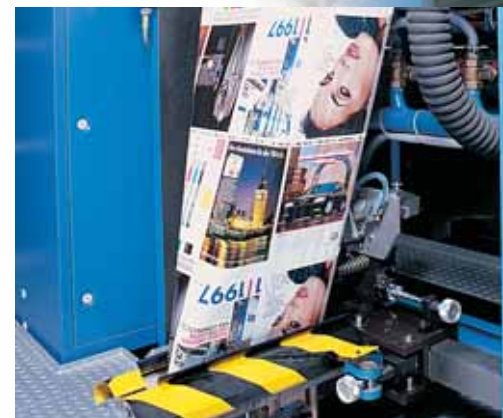
The position of the former section and the angle of the former nose are both adjustable
