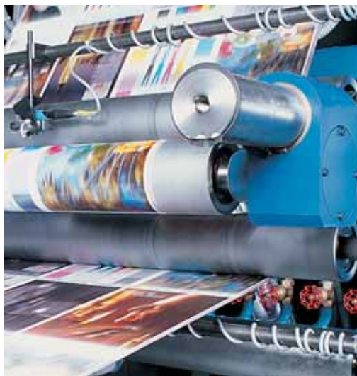
Measuring rollers monitor web tension
