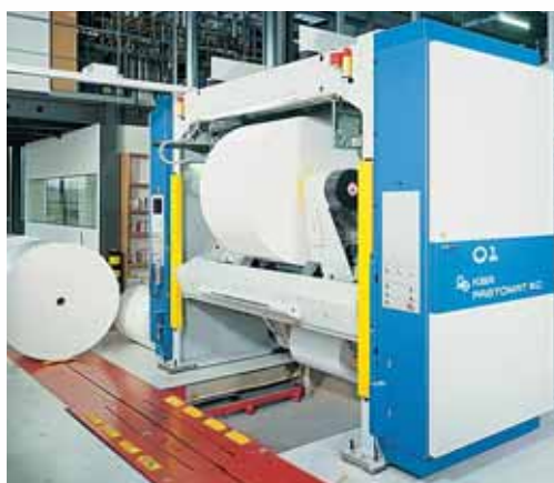
High-performance Pastomat RC reelstand for a maximum web speed of 15.2mps (2,992fpm)
