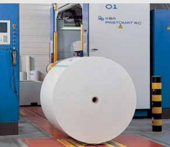
KBA Patras A delivers the prepared reels to the reelstands automatically
