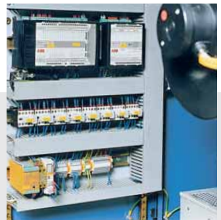
The drives are synchronised via an electronic (virtual) shaft
