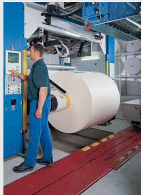
The display in the side frame presents important operating data and enables production parameters to be entered at the reelstand
