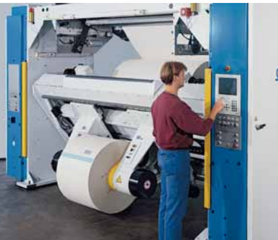
The standard features of the KBA Pastostar RC include motor-adjustable reel arms to handle reels of different widths
