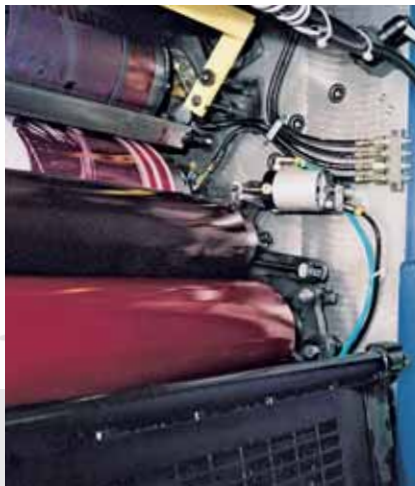
The printing unit can handle stocks of different thicknesses without the need to pack the blanket cylinder...
