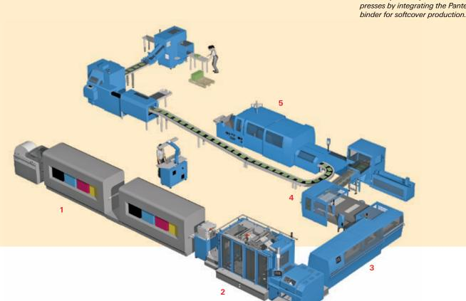
The SigmaLine digital complete system harnesses the impressive performance of inkjet printing presses by integrating the Pantera perfect
