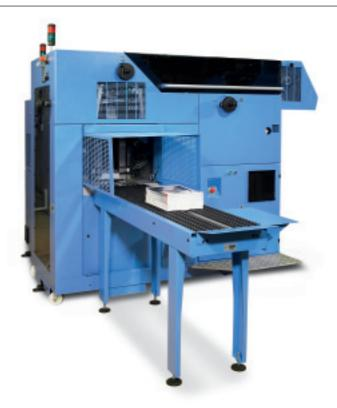
For gravure and web offset products The Listo is used for processing gravure and web offset products. After exiting from a press, bundles of trimmed and untrimmed stacked and layered print products are created inline and at full press speed, then stacked on pallets by an automatic palletizing system from Muller Martini. The Listo also works perfectly in offline trimming lines.
