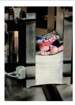
**Protective handling on the turntable** In the pre-stack unit, the products are supported by a linear guided fork. A layer lift transports the pre-stacked bundles to the turntable. The minimum product drop distance from the stack unit to the turntable unit guarantees perfectly centered and copyspecific layered and stacked bundles. Single and double production can be processed.
