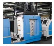
Digital Printing Unit Variable data can be printed in line at full machine speed by means of a digital printing tower that is easy to integrate.
