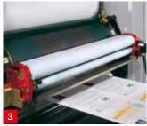
Blanket Wash-Up System As a standard feature, all printing units are designed to allow a blanket wash-up unit to be added.
