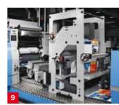
Register and Ink Control Automatic register control and in-line ink density control functions enable rapid setup times and optimum circulation stability.
