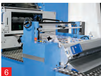
6 Register controller The scanning heads of the register controller are positioned immediately after the printing units to ensure fast reaction times.
