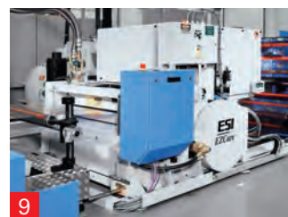
9 Electron-beam curing When manufacturing food packaging, the printing ink can be cured using electron-beam technology.
