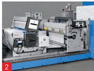
2 Web cleaning and corona treatment Before printing, the web is cleaned with or without a web contact and then treated with the corona station to improve ink adhesion.
