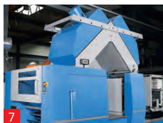
7 Flexo printing unit Infinitely variable sizes including servo drives, sleeve technology and an optional hot air dryer. For solvent-based, water-based and UV inks and lacquers.
