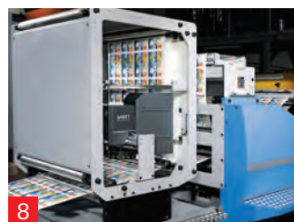
8 Web video monitoring Analog or digital web monitoring systems or a 100% print image inspection are used as required.
