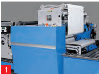
1 Infeed unit Depending on whether films or cardboard are being printed, one or two infeed rollers are used to guarantee stable web tension control.
