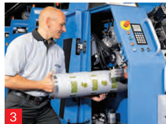
3 Offset sleeves Replacing the handy and cost-effective plate and rubber blanket sleeves offers infinitely variable print lengths.
