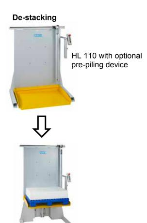
After the cutting material is de-stacked, lowering is carried out semi-automatically, i.e. the procedure is started manually, then automatically stopped after reaching the preset working height.
