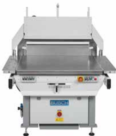
Basic position with pneumatic side flaps open
