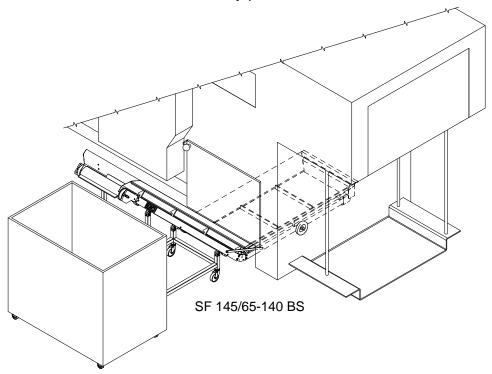
with one single conveyor into a container up to a height of 145 cm
