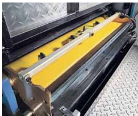
Swivelling ink ducts facilitate ink changes
