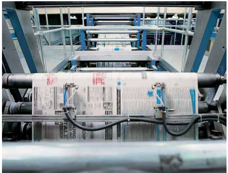
Left: The web running into the folder via the former, viewed from the dedicated AC drives for the draw rollers in the superstructure
