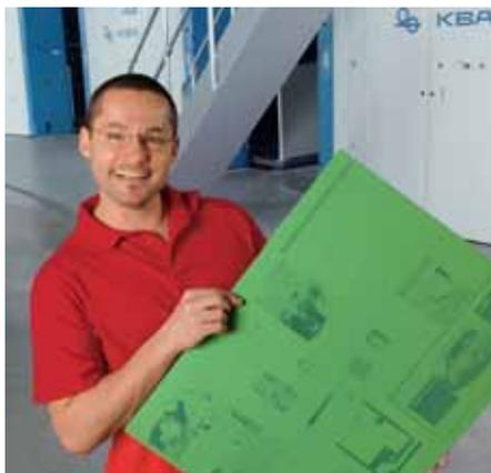
A service life of 120,000 to 150,000 cylinder revolutions is now the norm for waterless offset plates
