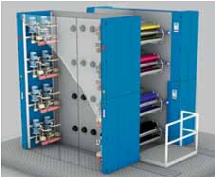
The TemperaTronic inking-unit temperature controls are integrated in the switch cabinets
